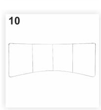
9. Add the five straight bars obtained at point 3 to one of the horizontal curved bars obtained at point 6, making sure to match the numbering / marking from the elements that join. 10. Add the second horizontal bar at the top of the system thus formed so that you'll get a complete frame. Now the PopUp structure is ready.
