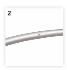
1-2. First join the aluminium tubes connected by elastic to form the support bars of the PopUp: insert each tube in its pair, press the button on one of the tubes and push one tube toward the other one provided with an orifice, as shown in Figure 1. When combined correctly, a "click" will be heard and the button will come out through the orifice, as in Figure 2.
